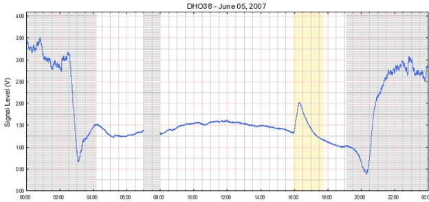
Figure 11: June 05-2007 measurements of DHO38. The grayed areas indicate approximately the periods of time during which events cannot be detected. They correspond to nighttime and to transmitter shutdown. The SID is highlighted in yellow.
