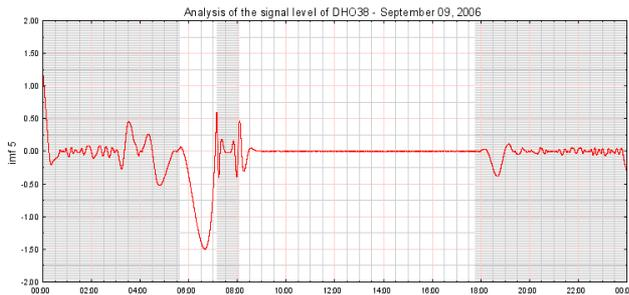
Figure 9: Evolution of IMF 5 component when taking into account the values recorded during the transmitter shutdown. The component remains close to zero during the day, except for the artifacts before 07:00 and after 08:00.
