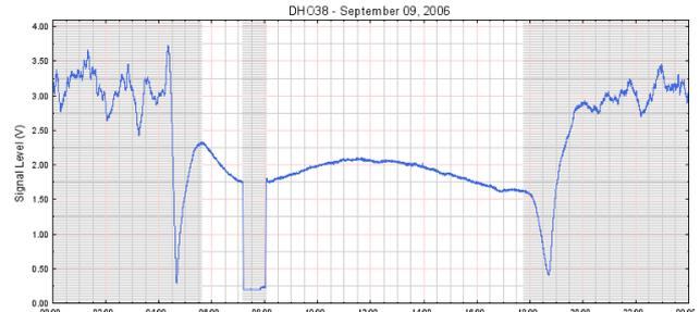
Figure 4: Typical example of the evolution of the DHO38 signal amplitude on a quiet day (September 09, 2006) with stable propagation during the day.
