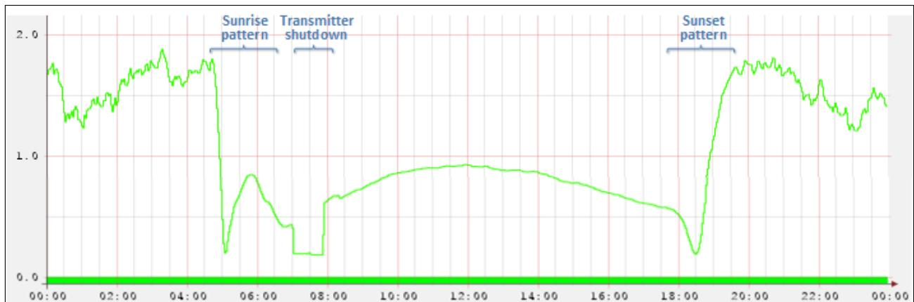
Figure 2: Typical evolution of VLF signal amplitude on a quiet day. The daytime propagation is very stable.
