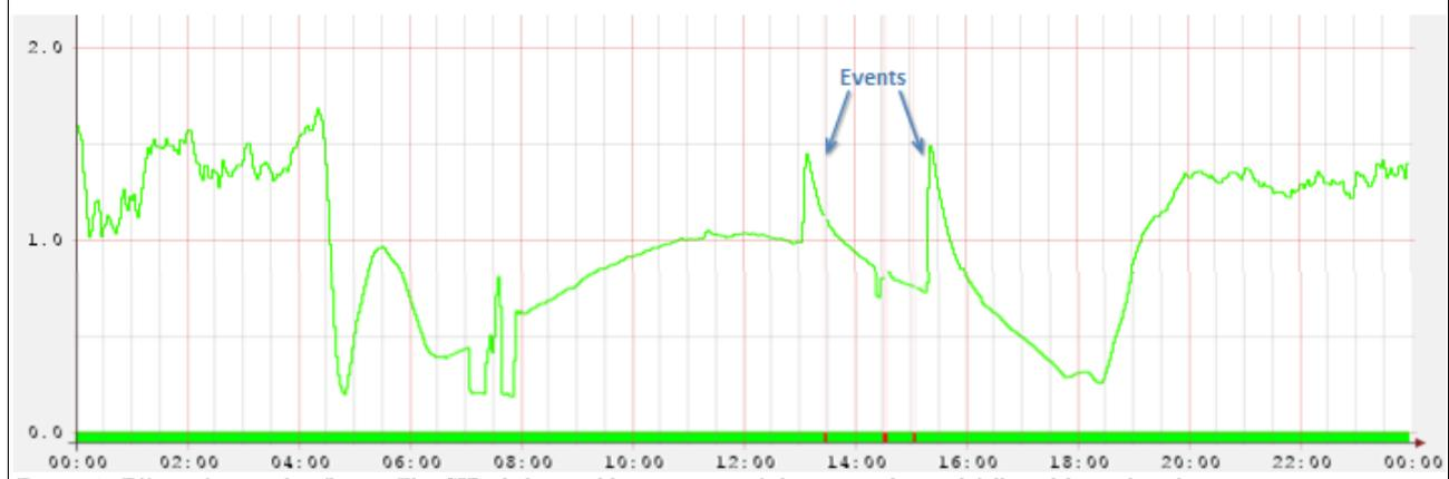
Figure 3: Effect of two solar flares. The SIDs led to sudden increase of the received signal followed by a slow decay.
