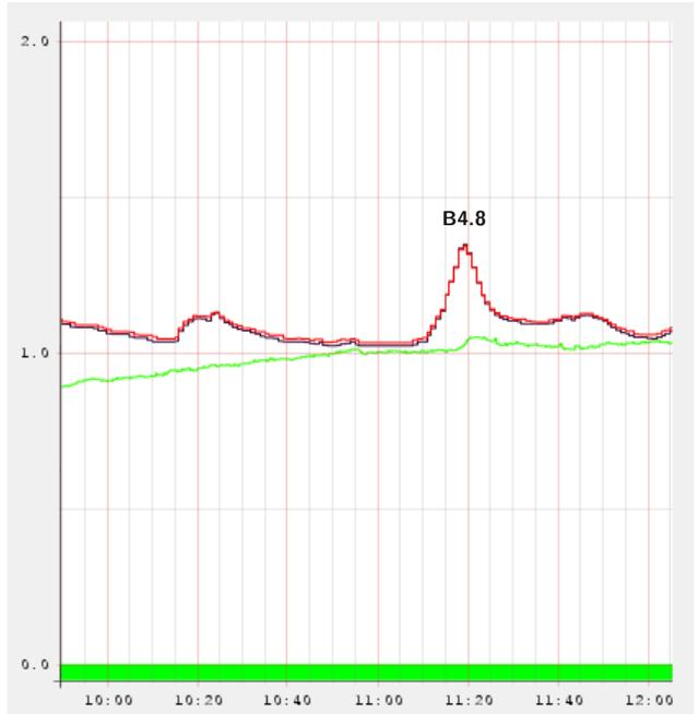
Figure 19: Detail of the DHO38 signal level during the B4.8 flare on April 05, 2006 and correlation with GOES measurements. x-axis is the UTC time, y-axis represent the measured signal level in volts. The signal measurement is the green plot. Purple and red plots are GOES10 and GOES12 measurements shown on a logarithmic scale. B-class starts at  $y=1.0$  and C-class starts at  $y=1.5$ .
