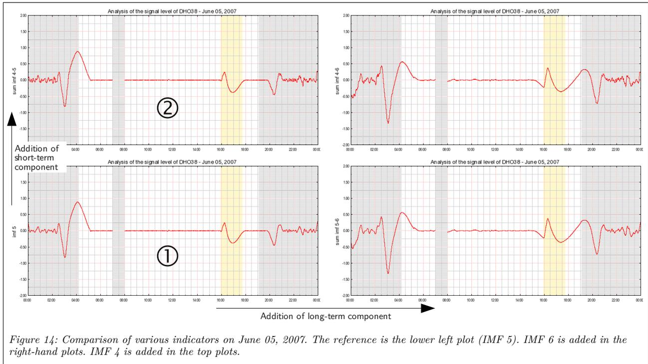
Figure 14: Comparison of various indicators on June 05, 2007. The reference is the lower left plot (IMF 5). IMF 6 is added in the right-hand plots. IMF 4 is added in the top plots.
