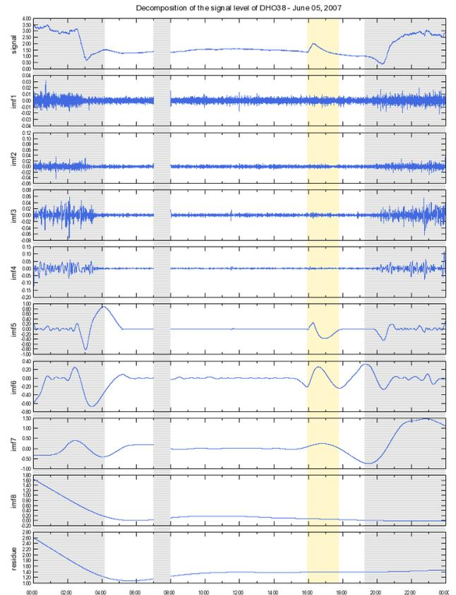
Figure 13: Components resulting from the EMD of the measurements made on June 05, 2007.
