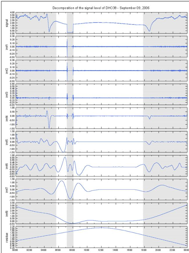
Figure 7: EMD Analysis of VLF signal strength. Each IMF represents lower frequencies than the previous one.
