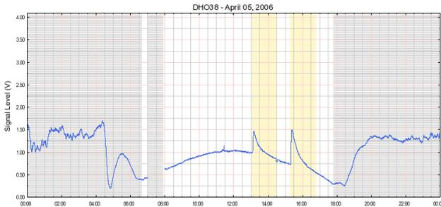
Figure 15: Signal amplitude of DHO38 recorded on April 05, 2006. Two events resulting from C2.6 and C8.1 x-ray flares have been recorded.
