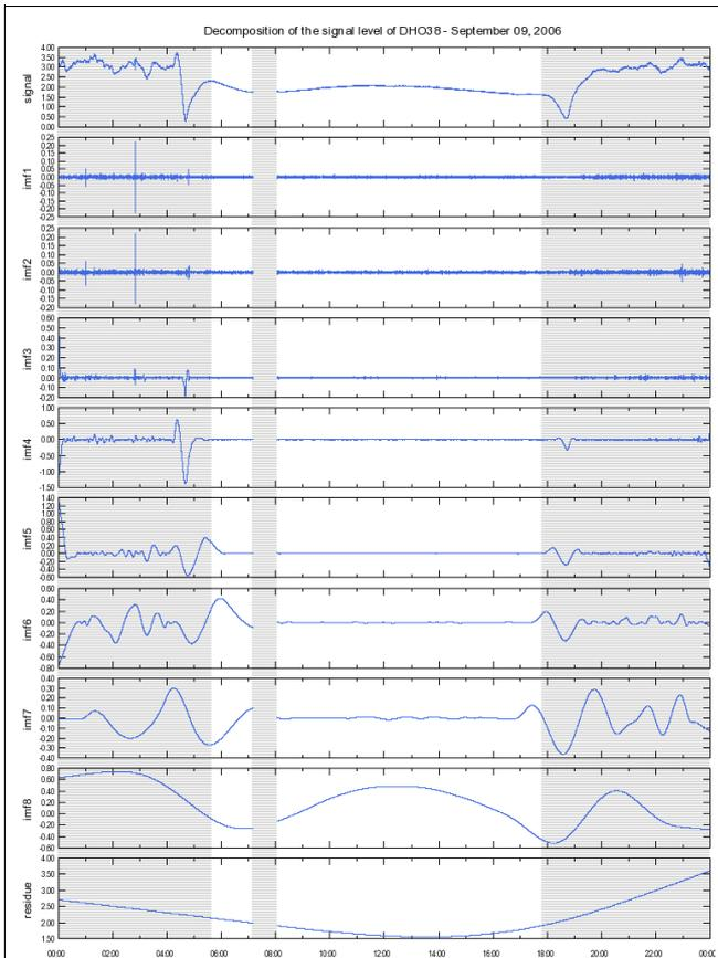
Figure 6: EMD of VLF signal strength when ignoring data recorded during the transmitter shutdown.
