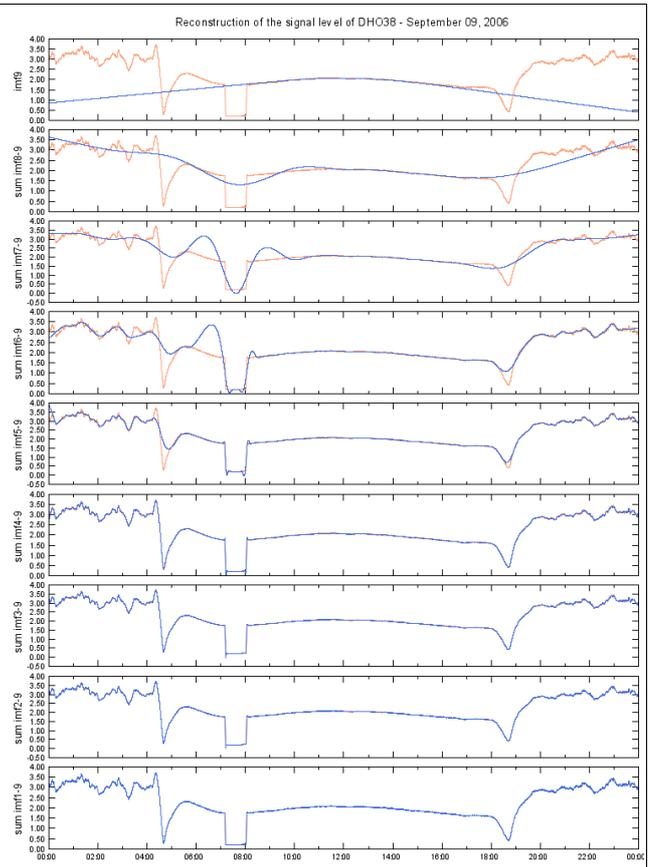
Figure 8: Reconstruction of the original signal by adding successively high-order to low-order IMF components.
