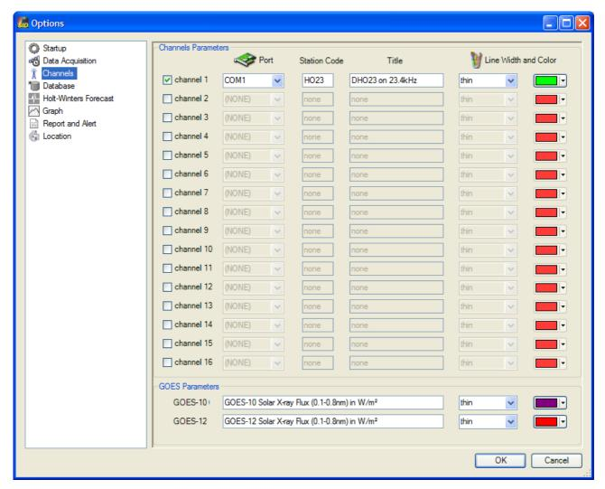
Up to 16 channels can be monitored by SID Monitor . This panel is used to select which channels are active.
