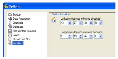
This panel is used to set latitude and longitude of station location. This information is used for sunrise, sunset and twilights time calculation. The sun position is stored in the database. SID events can only be detected during the day-time period.
