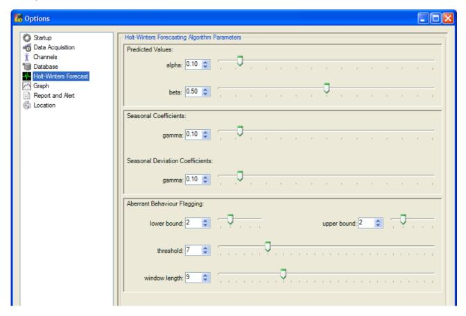
This panel is used to set all the parameters of the Holt-Winters aberrant behavior detection algorithm. More information on the effect of the various parameters is available in the Forecast FAQ.
