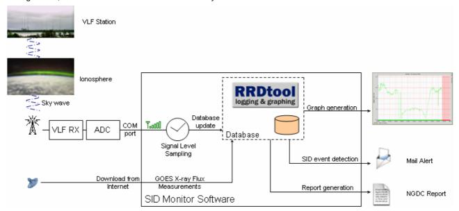
SID monitor acquires digital data from a VLF receiver. Up to 16 channels can be monitored simultaneously.
